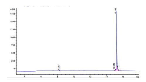
**Trace: HPLC Analysis of DPc10 Inactive Peptide**. Analysis carried out using 100 Å 4.6 x 50mm column, gradient from 0%-80% acetonitrile, in 8 minutes. Purity determined as 95%.
