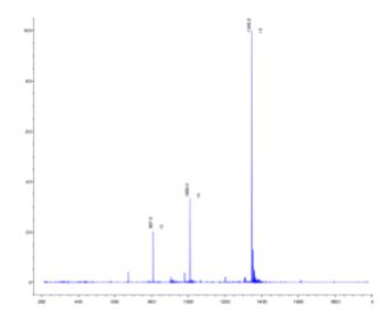
**Trace: Mass Spectrometric Analysis of Inactive DPc10 Peptide**. Molecular ion predicted: 4034.726 observed: 4034.1 [M+3H]. The range of molecular ions observed is due to the various multiply charged forms of the peptide ([M+3H], [M+4H], etc.).
