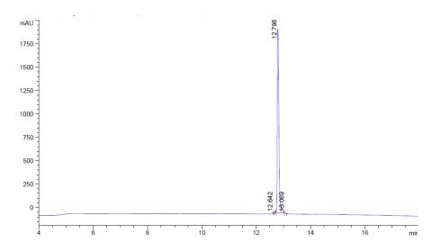
**Image: HPLC analysis of DPc10 Peptide**. Analysis carried out using 100Å 4.6 x 150mm column, gradient from 10%-90% acetonitrile, in 15 minutes. Dissolved in DMSO. Purity determined as 97.28%.
