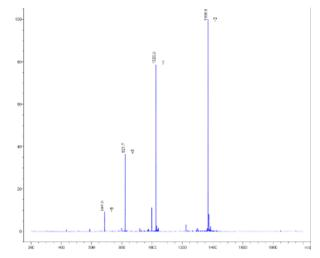
**Image**: **MS** Analysis of **DPc10** peptide. Molecular ion predicted: 4103.835 observed: 4103.835 ([M+3H]). The range of molecular ions observed is due to the various multiply charged forms of the peptide ([M+3H], [M+4H], etc.).
