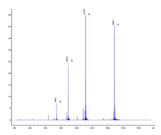
**Trace**: Molecular ion predicted: 4462.155, observed: 4461.3 [M+3H]. The range of molecular ions observed is due to the various multiply charged forms of the peptide ([M+3H], [M+4H], etc.).
