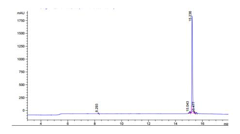
**Trace: HPLC Analysis of DPc10 Inactive Peptide**. Analysis carried out using 100 Å  $4.6 \times 50$ mm column, gradient from 0%-80% acetonitrile, in 8 minutes. Purity determined as 95%.
