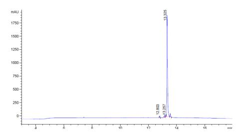
**Trace: HPLC Analysis of Fluorescein DPc10 Peptide.** Analysis carried out using 100Å 4.6 x 150mm column, gradient from 10%-90% acetonitrile, in 15 minutes. Dissolved in DMSO. Purity determined as 95%.
