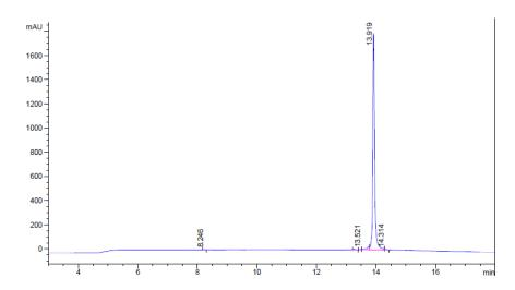
**Trace: HPLC Analysis of Fluorescein DPc10 Inactive Peptide.** Analysis carried out using 100Å 4.6 x 150mm column, gradient from 10%-90% acetonitrile, in 15 minutes. Dissolved in DMSO. Purity determined as 97%.
