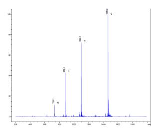
**Trace**: Molecular ion predicted: 4393.046, observed: 4392.6 [M+3H]. The range of molecular ions observed is due to the various multiply charged forms of the peptide ([M+3H], [M+4H], etc.).
