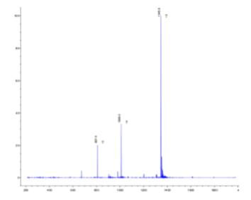
Trace: Mass Spectrometric Analysis of Inactive DPc10 Peptide. Molecular ion predicted: 4034.726 observed: 4034.1 [M+3H]. The range of molecular ions observed is due to the various multiply charged forms of the peptide ([M+3H], [M+4H], etc.).
